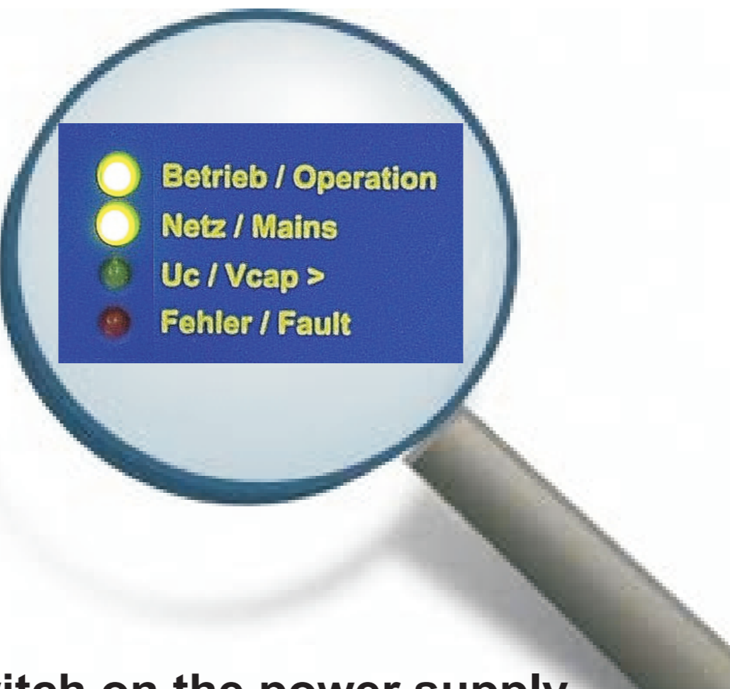
Switch on the power supply. The charging process starts. The LEDs „Betrieb/Operation“ and „Netz/Mains“ illuminate
