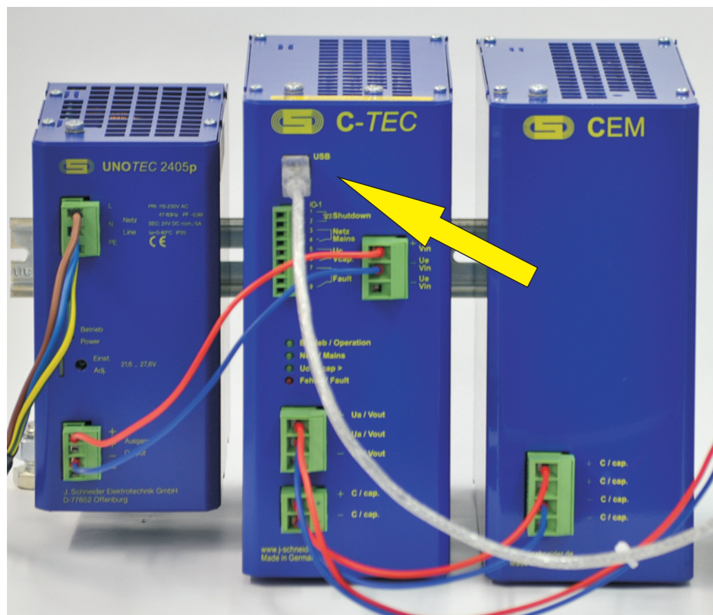
Connect the USB-cable to the PC (if present at the C-TEC)
