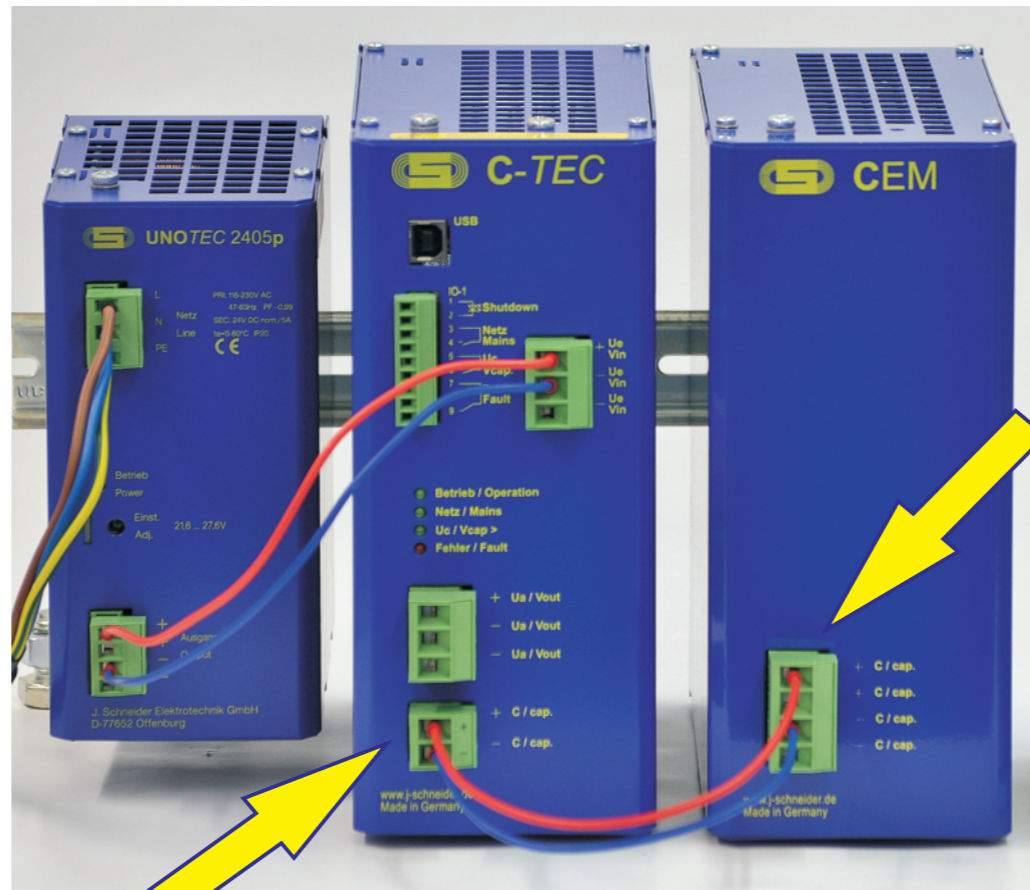
Connect the CEM to the capacitor output of the C-TEC
